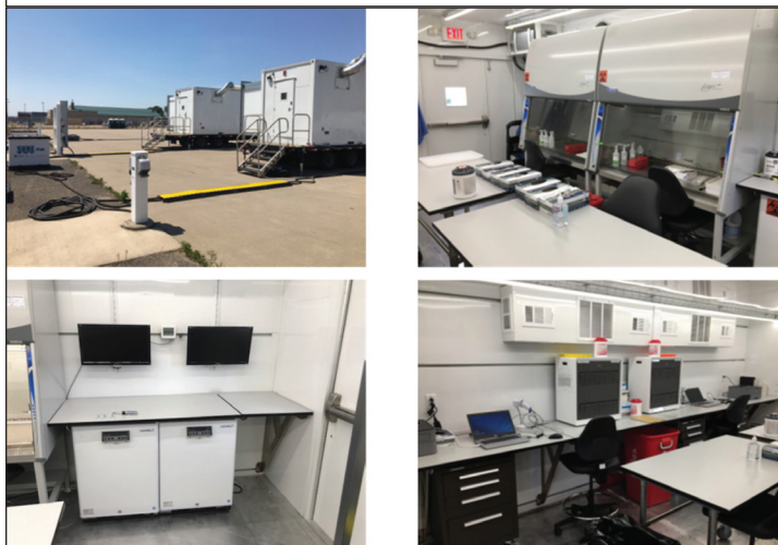
Figure 1. COVID-19 mobile molecular laboratory (MML) interior and exterior pictures. Physical establishment of the MML completed 48 hours after arrival at Camp Ripley Training Center, MN. Each laboratory had 2 biosafety cabinets, Cepheid GeneXpert Real-Time-Polymerase Chain Reaction (RT-PCR) instruments, and refrigerators/freezers.
